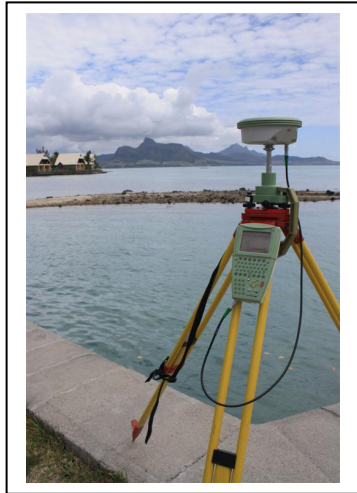
Figure 4. Example of Ground Control Points (GCP) utilised
