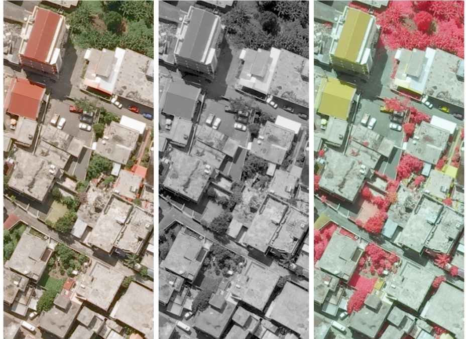
Figure 12. Natural RGB colour on the left, panchromatic in the middle and FCIR on the right
