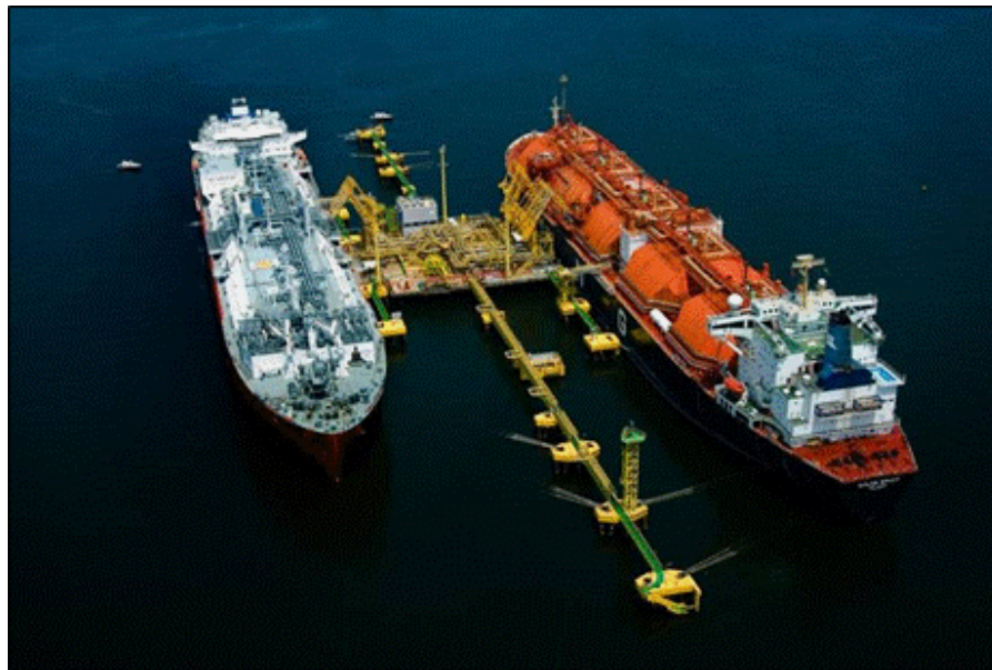
Exhibit 3-33: FSRU with Jetty Structure
