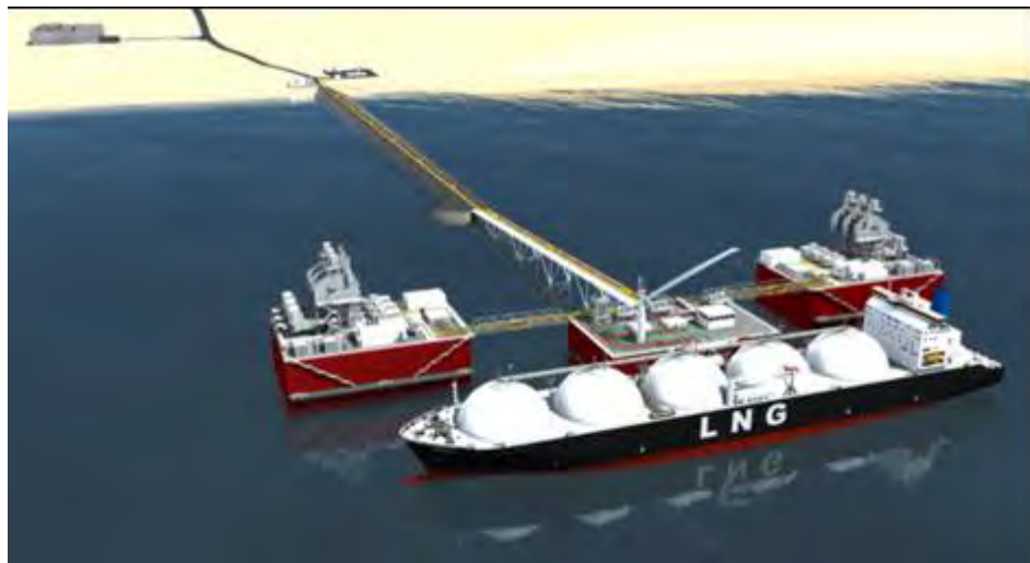
Exhibit 3-37: GraviFloat Storage Technology
