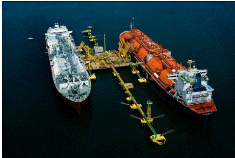
Exhibit 0-18: FSRU with Jetty Structure
