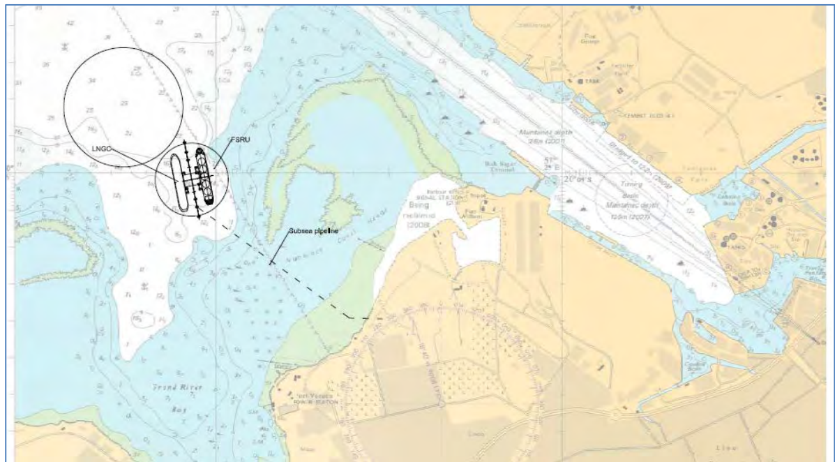
Exhibit 5-13 FSRU based LNG marine terminal
