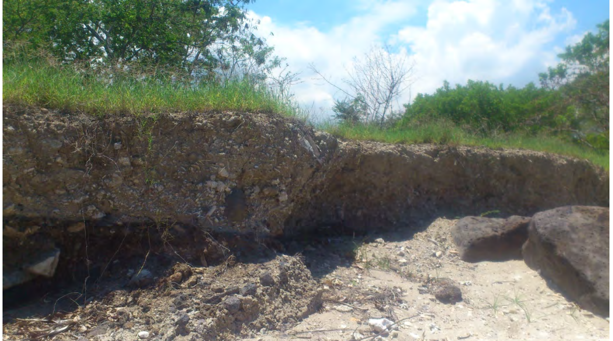
Exhibit 4-17 Photo taken at Les Grandes Salines nearshore site showing the top sandy-clayey stratum with presence of gravel and larger rock material.
