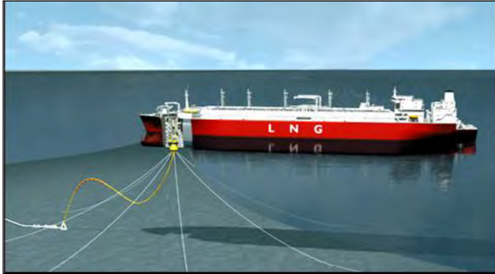
Exhibit 5-8 Disconnectable buoy mooring
